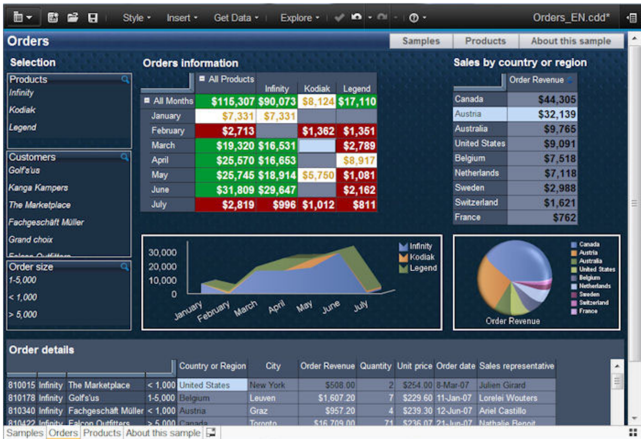
Figure 7. The Orders information crosstab showing different colored cells and text for the defined conditional styles
